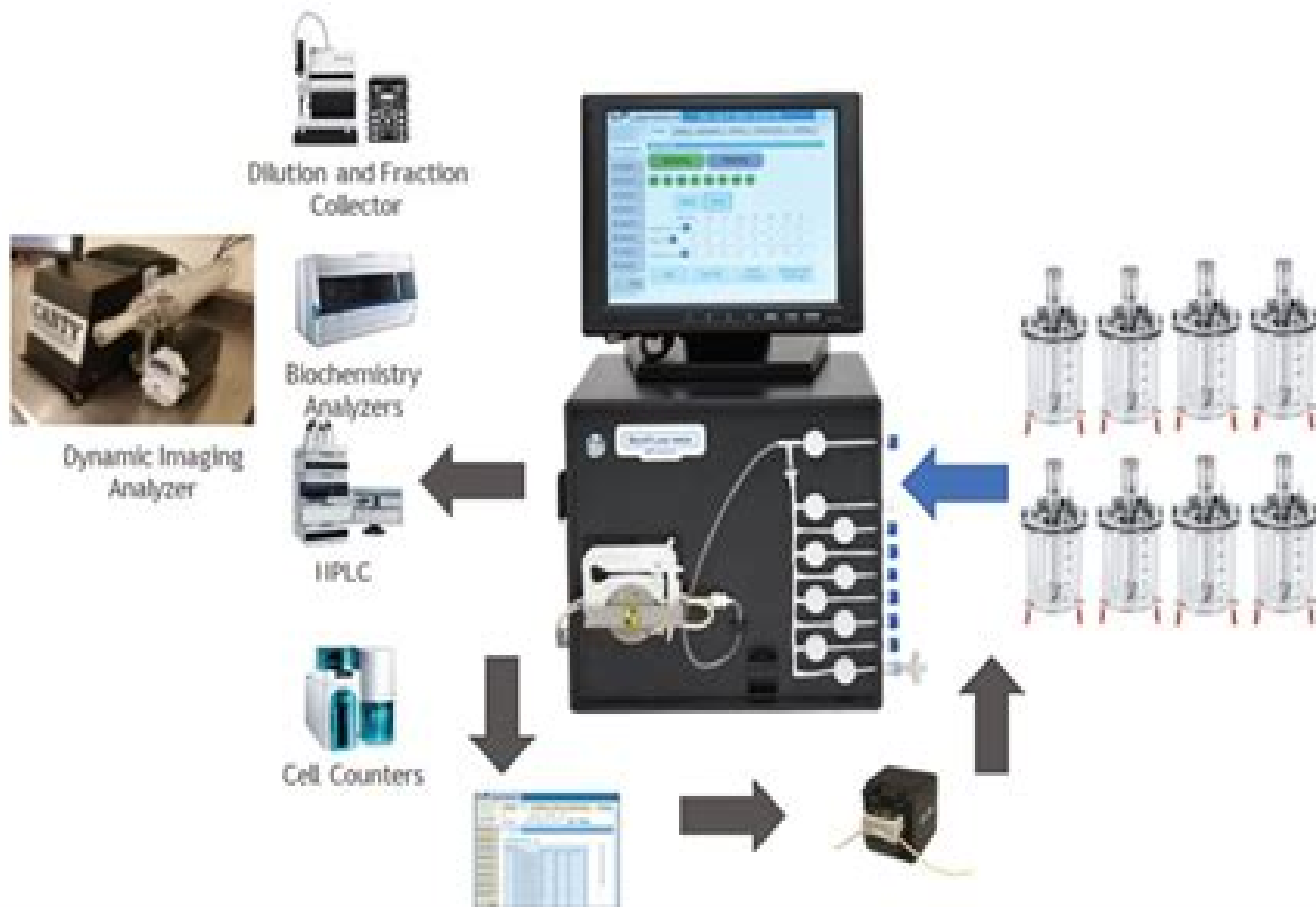
Figure 6. SegFlow™M autosampler interfaced with eight bioreactors delivering samples to off-line analytical equipment.
