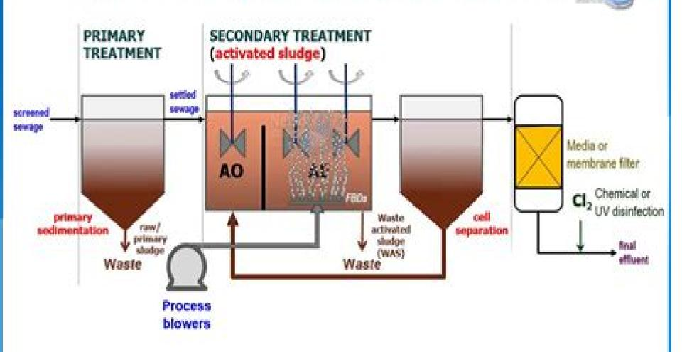
Treatment of Effluent with Aerobic Reactors
