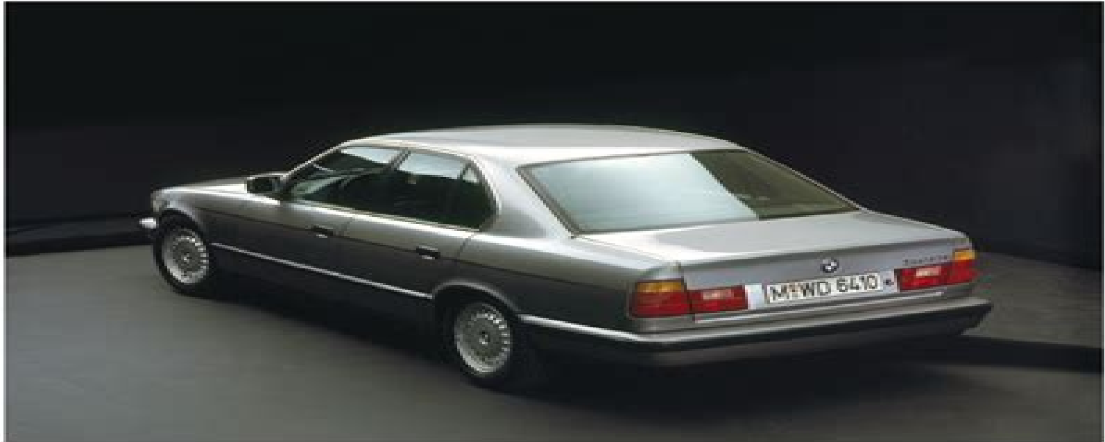
This rear overhead view of an early 520i shows very clearly how resolved the overall body shape was. Also apparent here are the 'Hofmeister kink' at the trailing edge of the rear door window and the two separate elements of the rear lights, which always lined up perfectly when the car was new.
